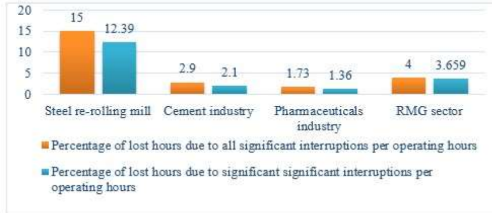
Fig-3: Percentage of lost operating hours due to five significant interruptions and sector wise significant interruptions.
